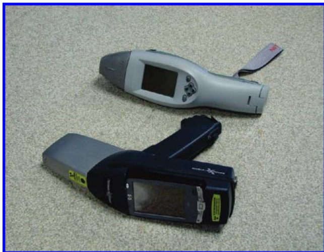
Figure 1. Picture of Niton XLi (top) and Innov-X \alpha -2000 (bottom) field-portable XRF analyzers.
